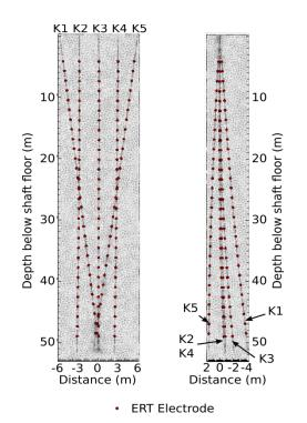
**Figure 6.1.** ERT computational mesh perpendicular to West Access Drift (left-hand figure) and parallel to the drift (right-hand figure) showing borehole and electrode locations in true dimension as derived from deviation logs. Note "shaft" should be "drift" in the axis labels.
