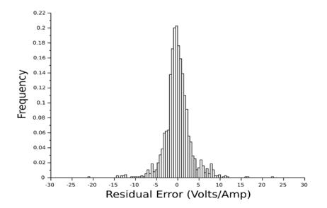
**Figure 6.3.** Weighted residual error histogram of baseline inversion data from the K1-K5 and K2-K4 planes corresponding to a normalized chi-squared value of 6.9.
