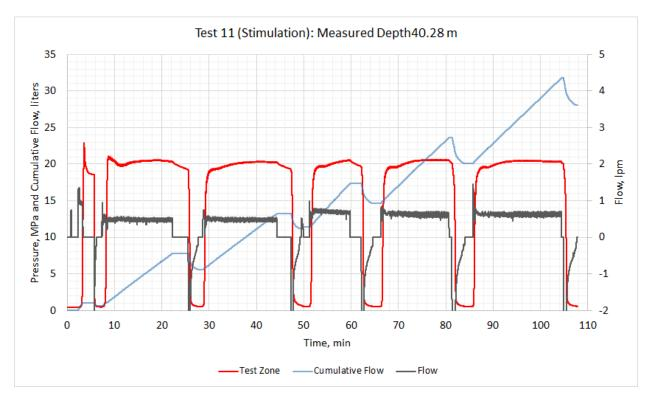
Figure 7.2. Pressure, flow, and cumulative flow for kISMET stimulation test.
