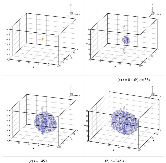
**Figure 4.5.** Induced fracture geometry at different times. The color scales with the hydraulic diffusivity (warm and cool colors = high and low hydraulic diffusivity, respectively). Notice that the initial large hydraulic diffusivity within the injection zone, and the trend of reducing hydraulic diffusivity (equivalent to crack aperture) from near wellbore to the crack front.
