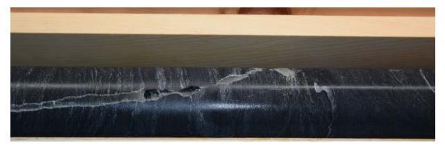
**Figure 2.13.** Open fracture encountered in kISMET-002 at ~91 ft (27.7 m). The fracture is lined with small quartz crystals, and is interpreted to be related to Tertiary-age mineralization.
