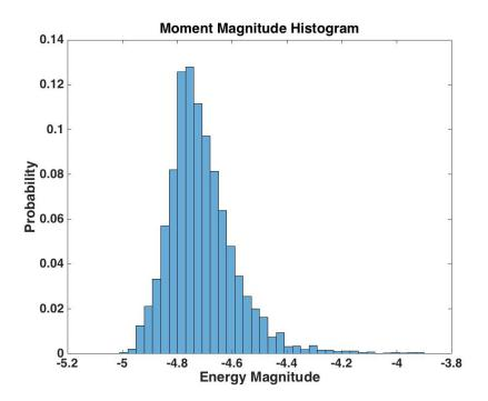
Figure 4.90. Histogram of the moment magnitude generated by the coupled network flow-DEM model.
