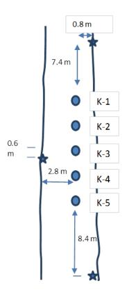
**Figure 6.4.** Arrangement of accelerometers (blue stars located in W, N, and S positions) with respect to the drift borehole geometry in the West Access Drift on the 4850L of SURF (Yates Shaft is toward the top of the figure). At this point only accelerometer (W) has produced usable data due to ambient noise in the drift. A geophone also was deployed in the K-2 borehole, where in this figure K-2, K-3, etc. = kISMET-002, kISMET-003, etc.
