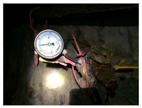
Figure 2.5. Instrumented drill hole with a static pressure of 700 psi (50 bars) at Drill Station 2.
