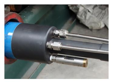
**Figure 5.5.** Top adapter on the straddle packer assembly shows the interval and the packer pressure lines and the normally-open relief valve. The parallel interval pressure line connected to the surface pressure transducer is hidden behind the stem connected to a wireline.
