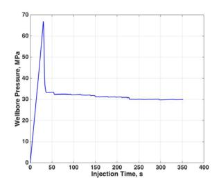
Figure 4.7. Wellbore pressure versus injection time.
