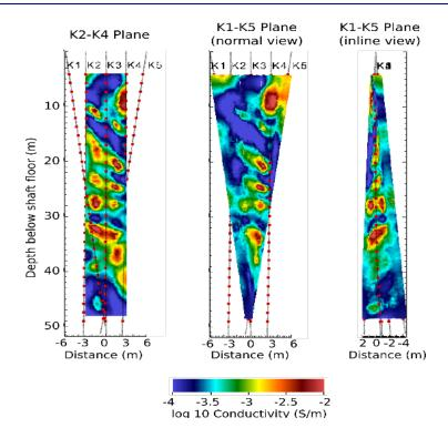
**Figure 6.2.** Baseline ERT inversion results. (Left-hand side), Bulk conductivity in the K2-K4 plane; (Center), Bulk conductivity in the K1-K5 "plane;" (Right-hand side), Bulk conductivity in the K1-K5 "plane" as viewed along the K2-K3-K4 plane from K1 to K5.
