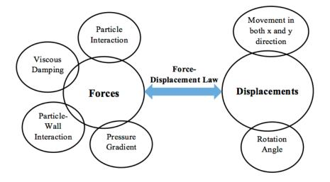
Figure 4.2. The algorithm of quasi-static DEM model.
