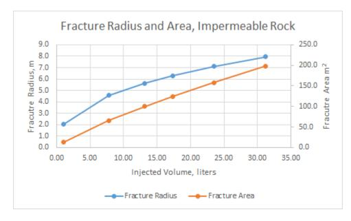
Figure 7.3. Fracture area and radius for impermeable rock.
