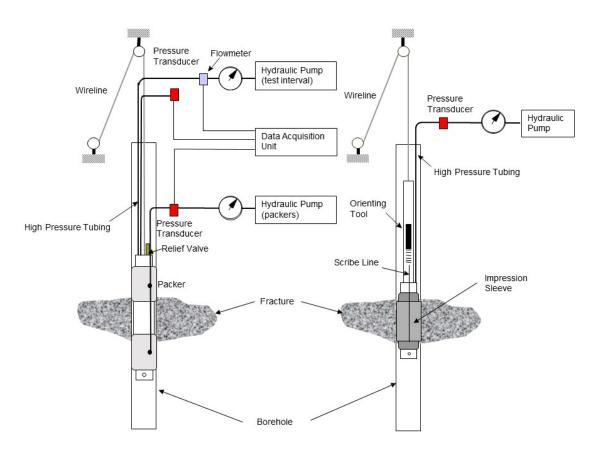
**Figure 5.4.** Wireline hydraulic fracturing system: Straddle packer for fracturing (left) and impression packer for fracture delineation.
