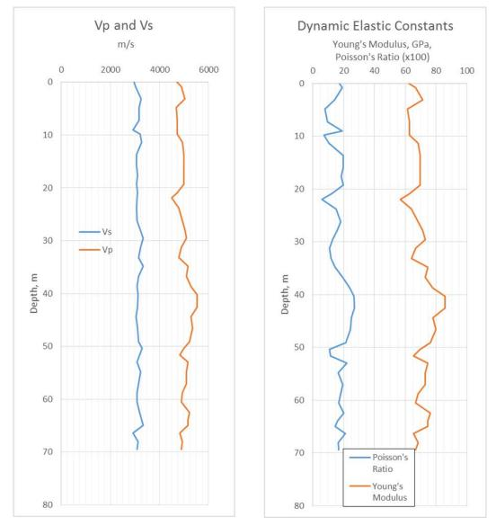
Figure 6.9. Preliminary full waveform sonic log for kISMET-003 with calculated dynamic elastic constants.
