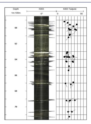
**Figure 6.6.** Portion of the kISMET-003 pre-test characterization log showing existing fracture and foliation conditions. In the optical image attribute plane, the markers indicate the dip directions of existing annealed fractures or foliations. The tadpole view on the right-hand side gives the quantitative values for all picked features with a confidence interval greater than 80%. No open fractures were readily apparent.
