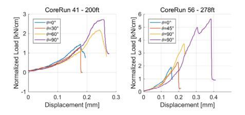
**Figure 3.6.** Load-displacement curve from Brazilian-disc tests on two groups of samples from cores recovered at 200 ft and 278 ft (61 m and 84.7 m) below the 4850L. The diametric load is normalized by the sample thickness to allow comparison.
