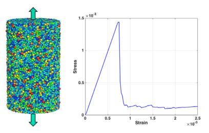
**Figure 4.3.** Numerical uniaxial tension test: (left) the DEM model used in the test (color scales with particle size) and (right) simulated dimensionless stress-strain curve for the uniaxial tension test.
