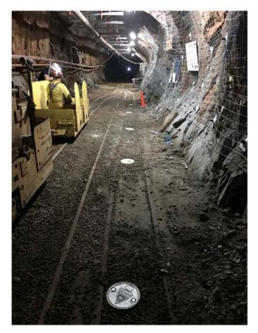
Figure 2.17. Five well "boxes" with white circular covers in the photo show well completion at the kISMET site in October 2016 after field experiments were completed.
