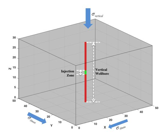
Figure 4.4. Simulated domain with a vertical open wellbore.
