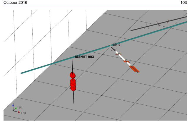
**Figure 8.3.** Visualization of hydraulic fractures and borehole breakouts. Rhyolite sections of borehole BH-3 are shown in white. For scale, borehole kISMET-003 is 100 m (328 ft) long. The end of Borehole D appears in the upper right (black terminating line subparallel to West Access Drift (aqua)).
