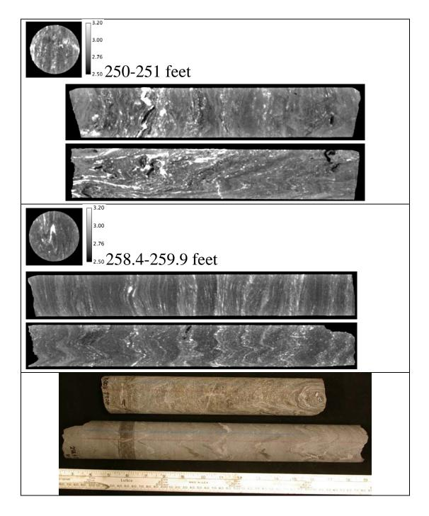
**Figure 3.1.** X-ray CT scans of core from 250-251 ft (~76.2 m) (top, Short" core) and 258.4-259.9 ft (~78.9 m) (center, "Long" core). Photographs of the both the "Short" and the "Long" cores are shown at the bottom.
