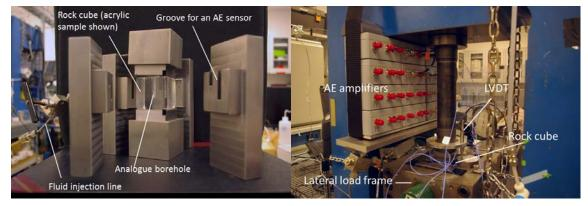
(a) Grooved loading platens for cube samples
