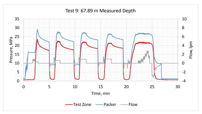
Figure 5.9. Pressure-time and flow rate-time plot obtained in Test #9 in kISMET-003.
