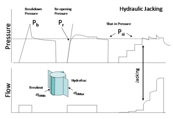
Figure 5.13. Idealized hydraulic fracturing pressure-time record. Inset shows location of triangular prismatic borehole breakouts relative to horizontal stress directions.
