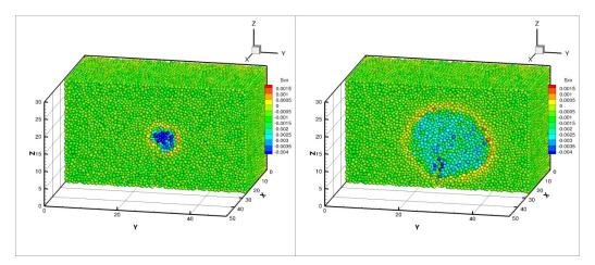
**Figure 4.6.** Dimensionless stress  $S_{xx}$  normal to the average crack plane during early (left) and (late) crack propagation stages.
