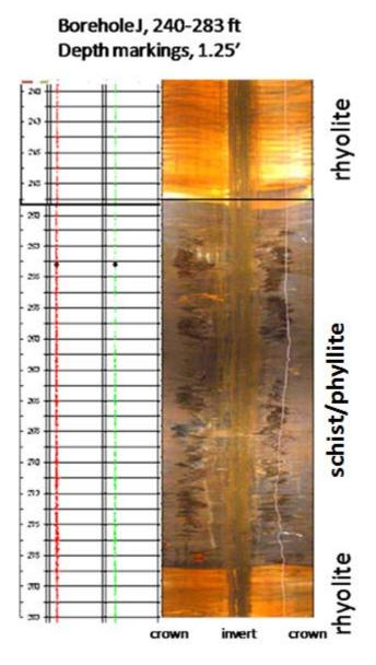
Figure 8.2. Borehole breakouts in DUSEL hole J.
