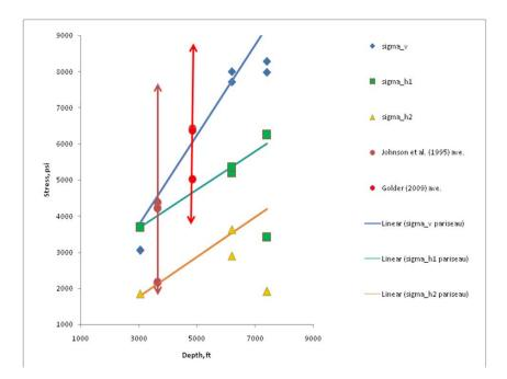
**Figure 5.2.** Legacy and recent stress magnitudes. The arrows at 3600 and 4850 ft (1097 and 1478 m) depth span the range of measured values while the symbols represent the averages for each principal stress.
