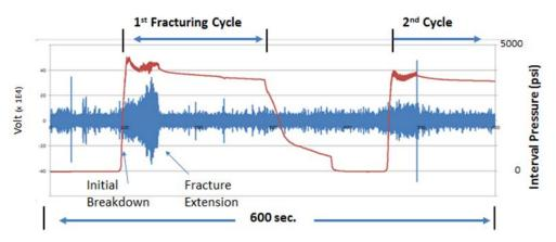
**Figure 6.5.** Seismic response detected by accelerometer W relative to fracturing pump pressure at a depth of 319 ft (97.25 m) from the borehole collar. The seismic data from the vertical channel were subjected to a bandpass filter between 290-310 Hz. The seismic response shows a good correlation with the pump pressure although seismic responses from fracturing at more shallow depths are not as well developed.
