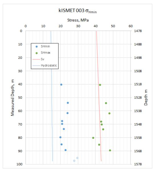
**Figure 5.14.** Minimum and maximum horizontal stresses versus depth in borehole measured and depth below surface. Vertical stress is based on a density of 2800 kg/m<sup>3</sup> and hydrostatic pressure is based on water column to the surface.
