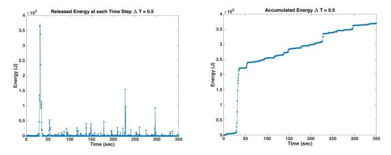
Figure 4.9. (Left) released energy vs. injection time and (right) cumulative released energy vs. time.
