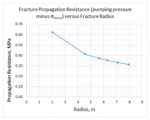
Figure 7.5. Propagation resistance versus radius
